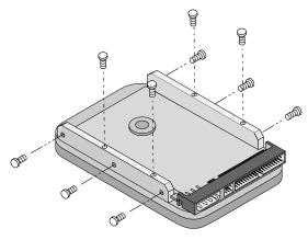
3 Slide the drive carefully into the drive bay. Secure the drive with four 6-32 UNC-2A mounting screws in either the side-mounting holes or the bottom-mounting holes. Do not over-tighten the screws. The screws should be inserted no more than 0.22 inch into the bottom mounting holes and no more than 0.14 inch into the side mounting holes. Do not use metric screws.
